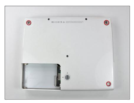
Remove the three newly-revealed Phillips screws.
