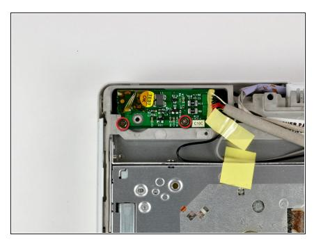
Remove the two Phillips screws securing the DC-In board, removing tape as necessary.
