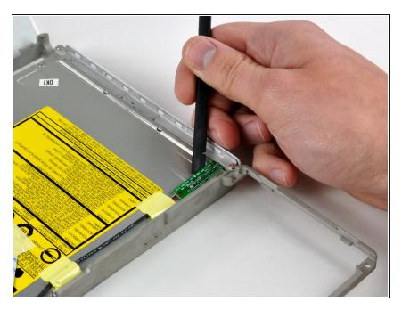
Use a spudger to pry up the Reed Switch Board from the optical drive, removing tape as necessary.
