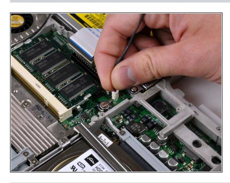
Use your fingers to disconnect the Reed Switch Board connector from the logic board.
