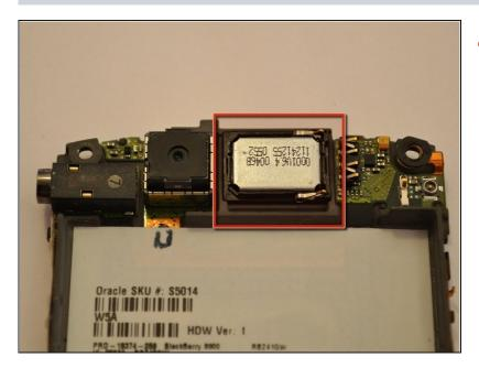
Replace the entire center piece of the case to replace the speaker.
