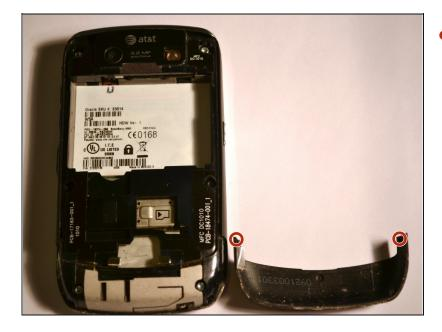
Remove the lower rear cover, using a small iFixit opening tool.
