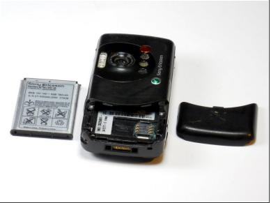
• Lift the bottom of the battery away from the phone with your thumb and rotate until the opening in the bottom of the case is oriented downward. The battery should slide out.
