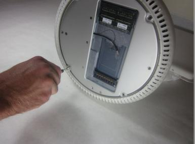
Remove the four 25mm T-15 screws.
