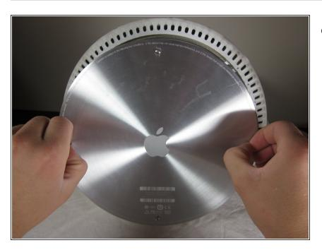
Carefully remove the base access panel.
