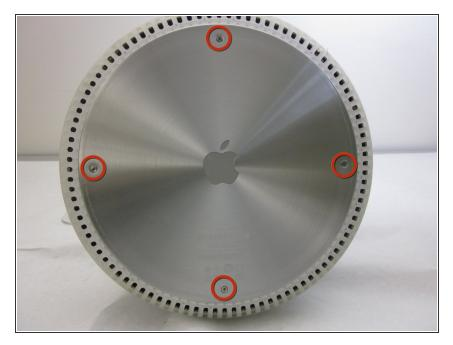
Loosen the four Phillips #0 screws.
