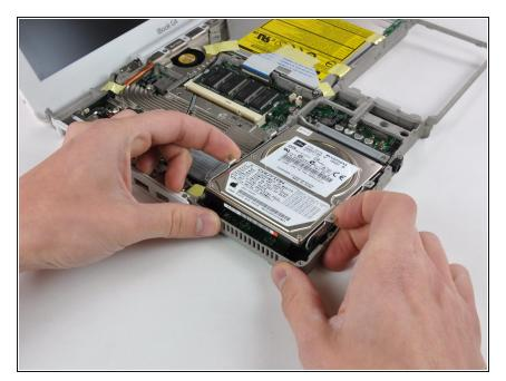
Slightly lift the hard drive from the free end and pull the hard drive straight away from the connector.
