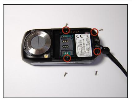
Remove the four 6mm screws behind the battery.
