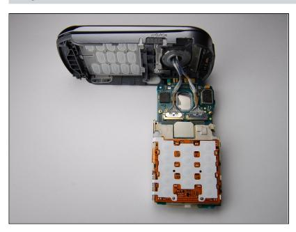
Once you have removed the back cover, use the plastic opening tool to carefully pry out the circuit board.
