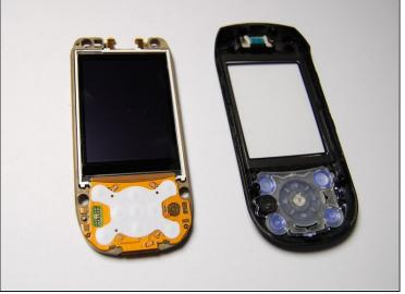
• In order to remove the LCD screen, use the plastic opening tool to pry the plastic piece from the LCD. Perform this step carefully to avoid scratching the glass screen.
