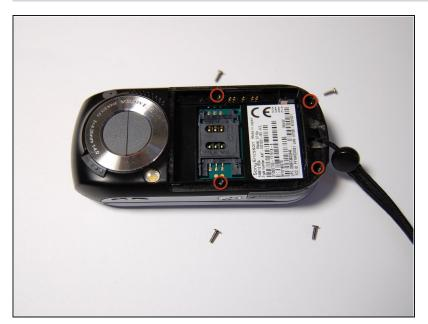
Remove the four screws using a Phillips #00 screwdriver.
