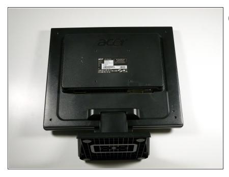
(i) Lay the monitor on a flat surface so that the back is facing up.
