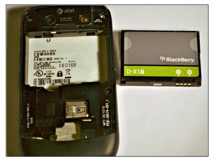
Remove the back cover and the battery from the device.
