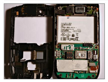
Separate the midframe from the rest of the device.
