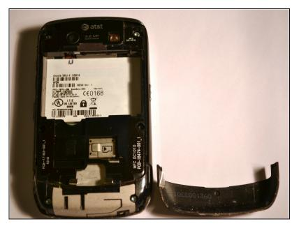
4 screws should be visible. Pry off the lower portion of the back to reveal all 6 screws.
