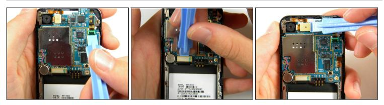
• Use the plastic opener tool to detach the three ribbons on the motherboard.
