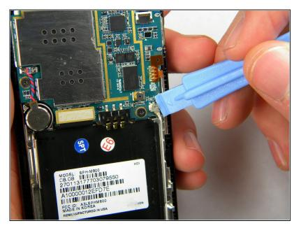
• Using the plastic opener tool, squeeze gently on the antenna cable connector and lift to remove the connector from its position.
