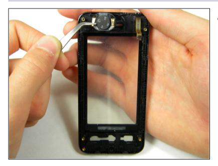
• Using <u>tweezers</u> to grasp the pins of the speaker, gently lift the speaker up out of its setting in the front case.
