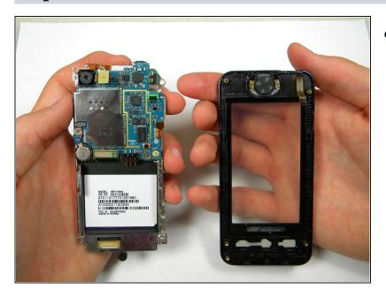
After removing lifting up on the motherboard, the front casing and center frame should be separated as shown.
