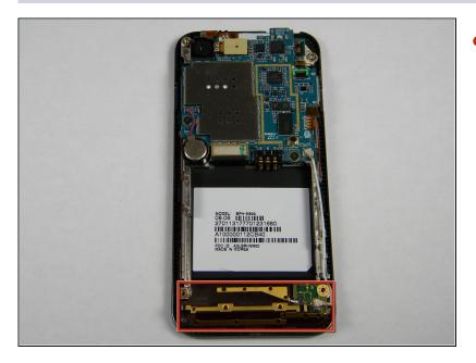
• With the screws removed, locate the antenna.
