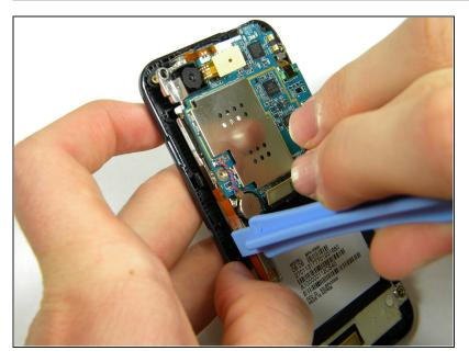
• Lift the motherboard away from the front casing.
