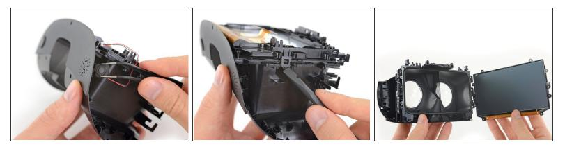
What we thought might be a wee speaker grille is actually for a sizable microphone mounted under the visor.
