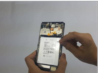
Remove any adhesive strips holding the battery in place gently using a fingernail or spudger.
