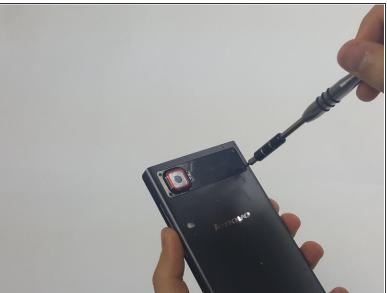
Remove the 4.9 mm torx head screws located on the camera plate on the back of the phone
