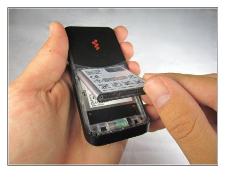
Lift the battery out from the bottom edge.
