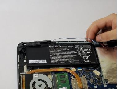
• Use the nylon spudger to pry away the blue/white wire that is positioned near your battery.
