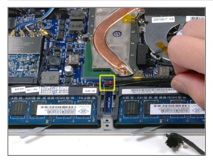
• Use a spudger to disconnect the right speaker connector from the logic board.
