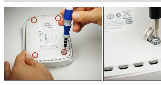
Unscrew the four 11.8 mm T-8 torx screws from the bottom of the router.
