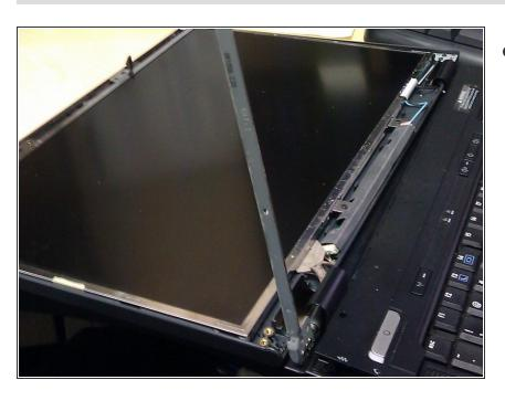
Place the new hinge assembly in and replace all screws.
