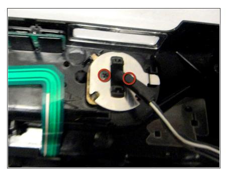
Remove (2) screws from viewfinder mount and electrical connecter, gently remove viewfinder unit from side cover.
