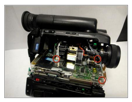
Remove (3) electrical connecters in order to pull side cover away from camcorder to expose back side of viewfinder.
