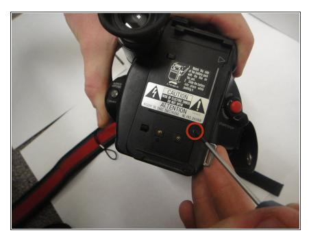
Remove battery terminal screw.
