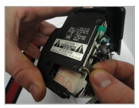
Pull battery terminal plug from camera.
