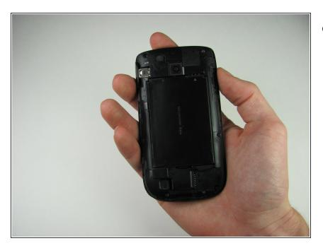
First remove the back cover of your phone to expose the battery.
