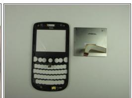
Using the Plastic Opening Tool, pry out the LCD screen and remove with fingers.
