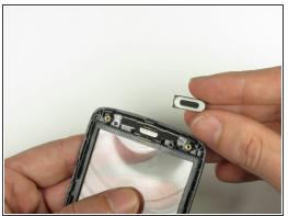
Use the Plastic Opening Tool to remove the internal ear speaker.
