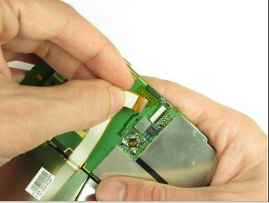
Gently pull on the ribbon cable to separate the motherboard.
