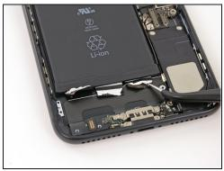
Peel back the three adhesive strips on the lower edge of the battery.
