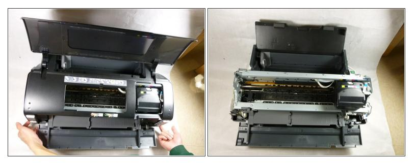
• Remove the upper housing by lifting it upwards.
