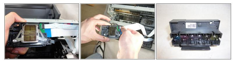
• Disconnect the two ribbon cables on the back of the printhead.
