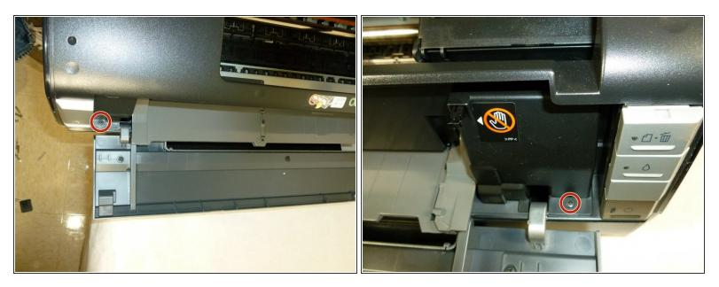
• Remove the two 10 mm Phillips #2 screws on the front of the printer.
