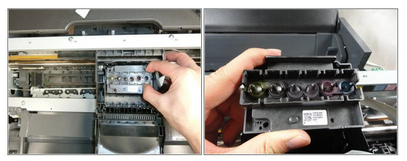
Remove the printhead from the carriage unit by lifting it up vertically.
