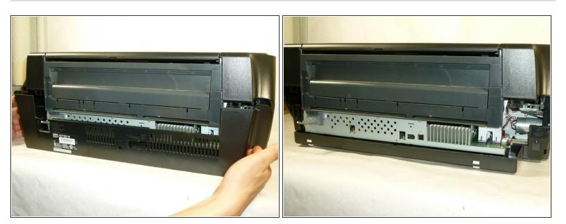
• Remove the rear housing by pulling it backwards.
