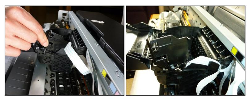
• Slide the cover upward and rotate it around the hinge by 90°.
