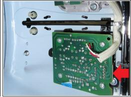
• The connector from the main platine to the switch platine.
