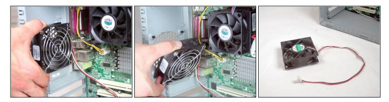
• Remove the fan from the case by pulling it towards the front of the device.
