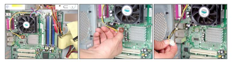
Remove the 4 pin ATX power connector from the motherboard by pressing down the holding latch and pulling out towards the side of the device.
