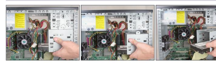
• Fully remove the hard drive cage by sliding it towards the back of the device and pulling down.
