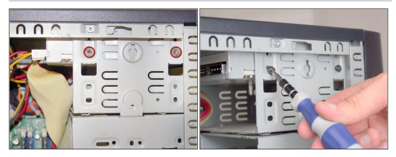
• Remove the 2 Torx T15 screws holding the optical drive in place.
