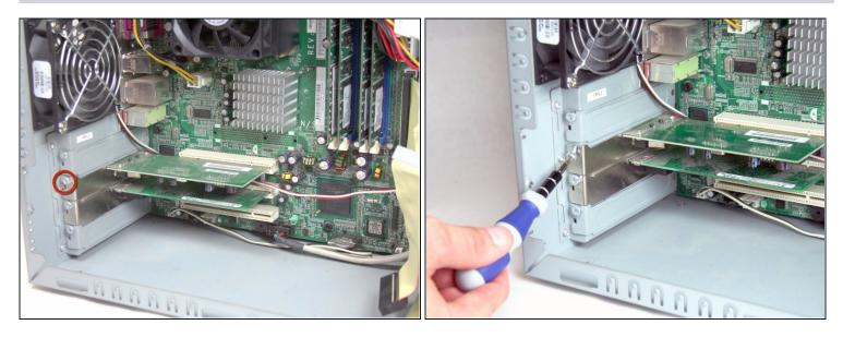
• Remove the Torx T15 screwdriver holding the PCI card in place.
