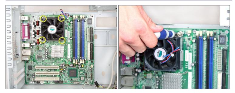
Unscrew the 4 Torx T15 screws holding the CPU Cooler in place.
