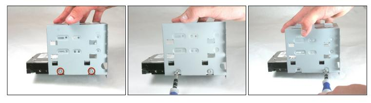
• Remove the two Torx T15 screws holding this side of the hard drive in place.
