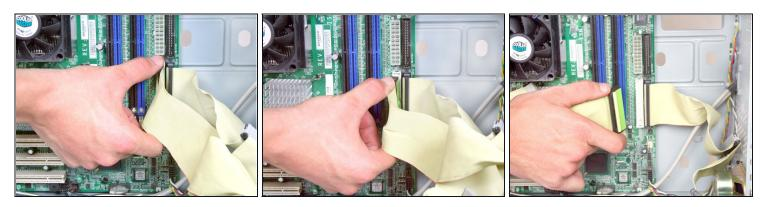
• Remove any IDE cables from the motherboard by pulling them out towards the side of the device.
