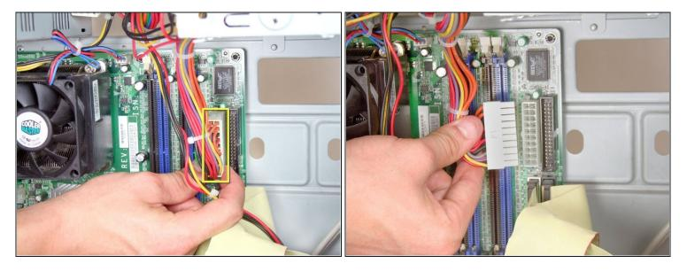
Remove the 20 pin ATX power connector from the motherboard by pressing down the holding latch and pulling out towards the side of the device.
