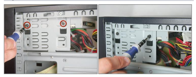
• Remove the other 2 Torx T15 screws holding the other side of the drive in place.
