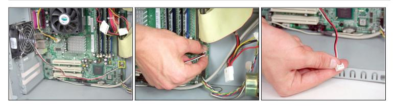
• Remove the 3 prong power connector from the motherboard by pulling it outwards toward the side of the device.
