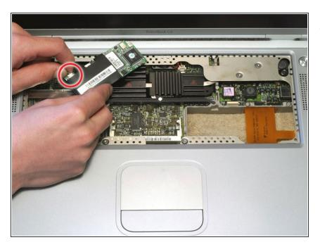
Disconnect the connector cable from the modem.
