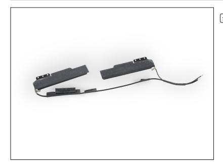
The Wi-Fi antennas are connected to a common ground via conductive tape.
