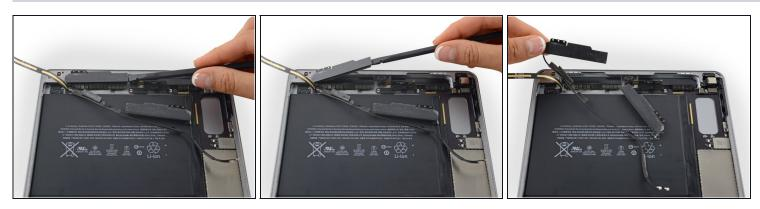
• Lift the left Wi-Fi antenna out of its housing and remove it.
