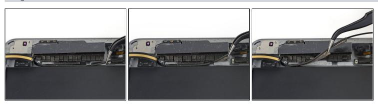
• Peel up the two remaining pieces of grounding tape attaching the left antenna to the rear case, as done in the previous steps.
