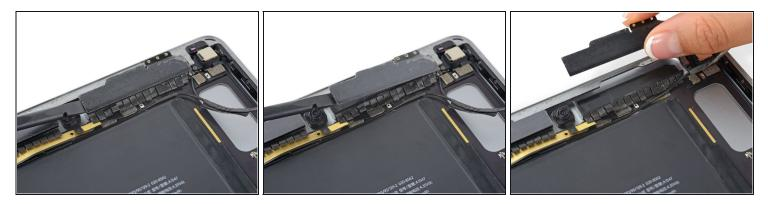
• Lift the right Wi-Fi antenna out of its housing and remove it.
