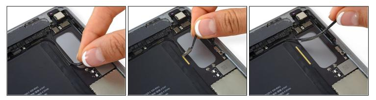
• Firmly grasp the antenna cable and peel up the grounding tape attaching it to the motherboard.
