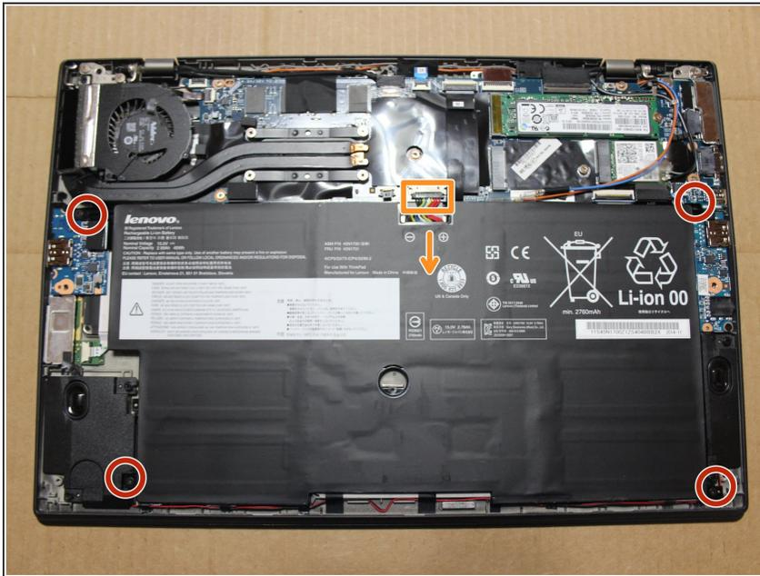
**⚠ Only use plastic to remove battery connector**
