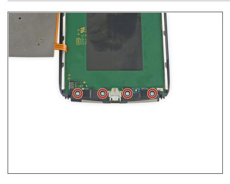
Remove the four Torx T5 screws securing the lower antenna board to the motherboard.
