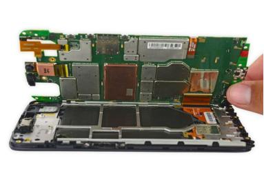
Carefully lift up the motherboard to expose the display connector.
