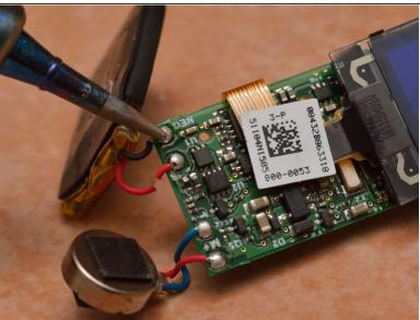
The Fitbit is very light and hard to hold, so it is recommended to tape the board in place when soldering.
