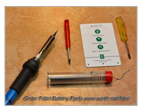
You'll need some plastic bits to separate the band, plus a torx driver, new battery and a soldering iron.
