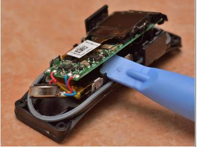
Once removed, there are 2 torx screws holding the circuit board in place. Remove these, and carefully pry the board out
