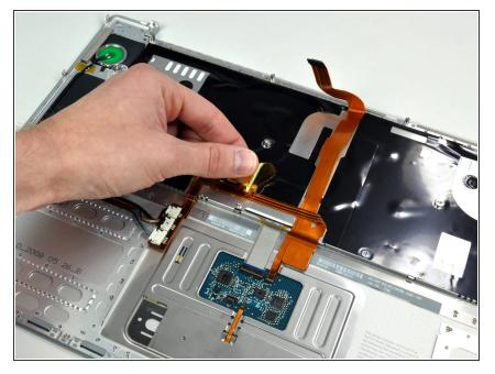
• Peel up the orange tape covering the keyboard backlight connector.
