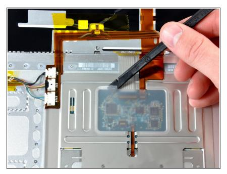
• Use a spudger to pry up the translucent plastic sheet covering the keyboard connector.
