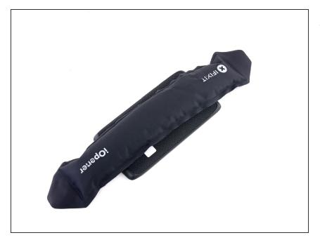
Prepare an iOpener and lay it over the rear case to soften the adhesive on securing the rear case to the phone.
