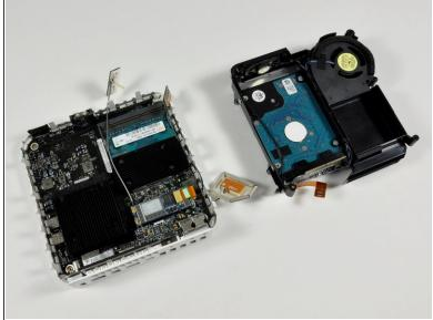
On the left we have the bottom housing, which includes the logic board, CPU, and RAM. On the right is the internal framework, which contains the SuperDrive, fan, and hard drive.
