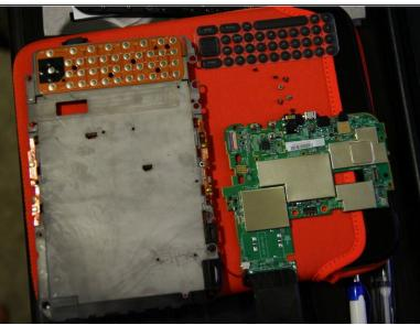
Once you've removed all the screws shown in step one, the PCB can be easily removed, along with the back plate.
