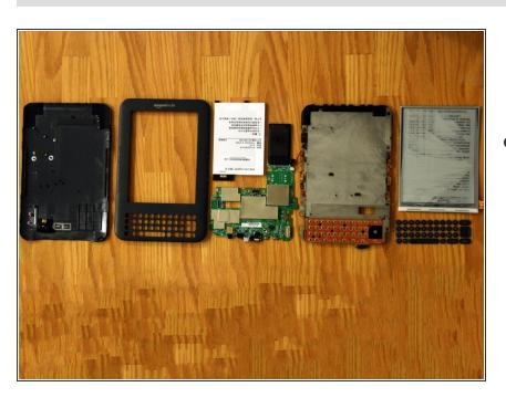
And there you have it. Very easy to disassemble but most of the parts are not replaceable, except for the screen and battery. To reassemble your device, follow these instructions in reverse order.
