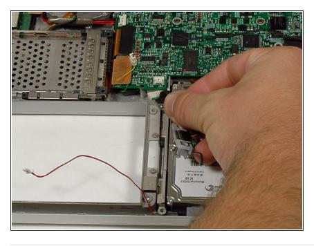
Disconnect the battery connector from the logic board.
