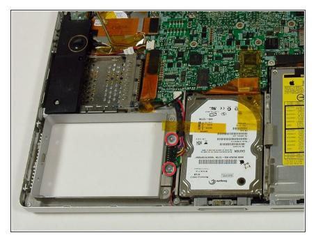
Remove the two Phillips screws securing the battery connector.
