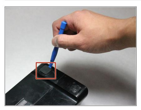
Use the plastic opening tool to remove the four rubber pads from the bottom of the device.
