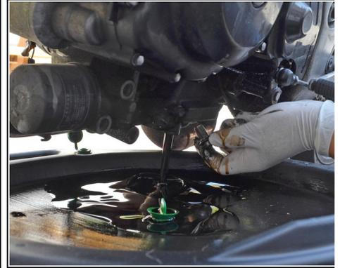
**⚠** Always wear protective gloves and eyewear when working with motor oil. Be careful if your bike has been running recently as the engine and exhaust may be very hot. Keep rags or towels nearby to wipe up any spills.
