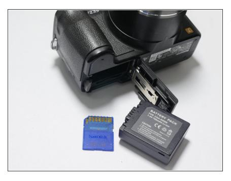
• Remove the battery and memory card from the unit.
