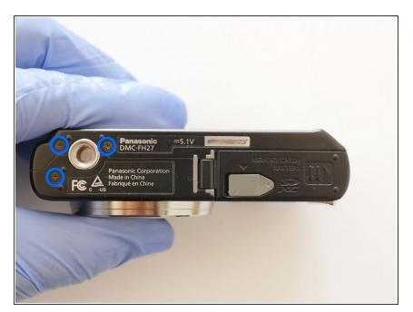
• Remove 3 (0.4mm) screws from the base of the camera.
