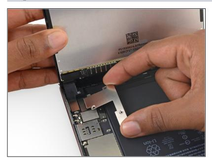
• Remove the battery/display cable bracket.
