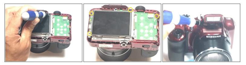
• Remove four 1.2 mm Phillips #00 screws from the top panel.
