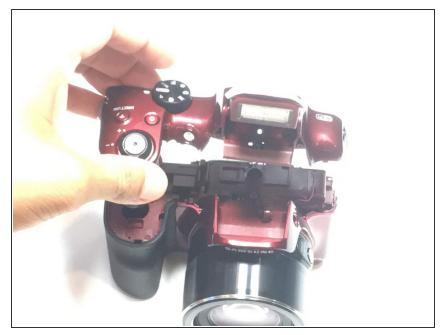
Using the flat end of a spudger, loosen the connection between the top panel and the device. Remove the top panel using your hands.
