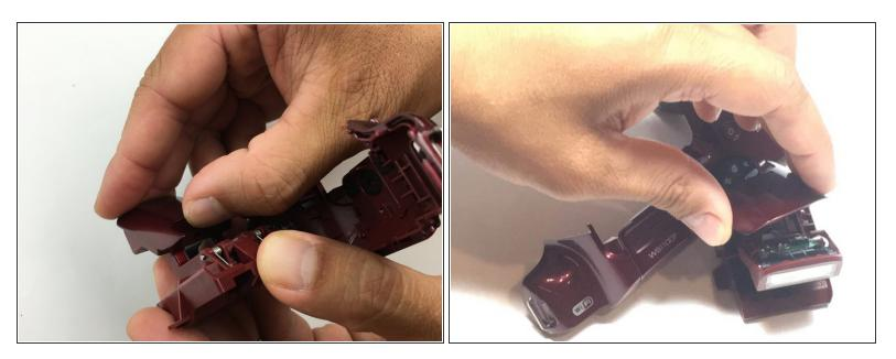
Using your hands, remove the top flash panel by pressuring down on the back to release a locking tab.
