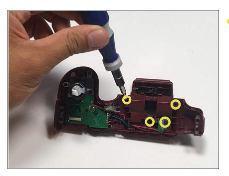
Remove four 1.2 mm Phillips #00 screws from the flash assembly
