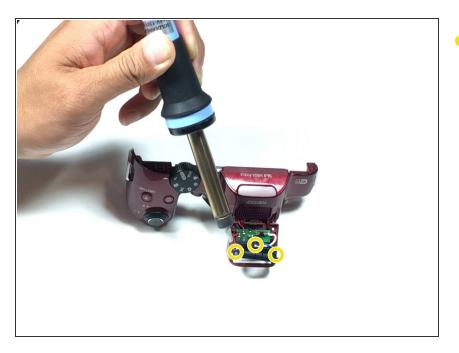
• <u>Desolder</u> three wires on the flash assembly.
