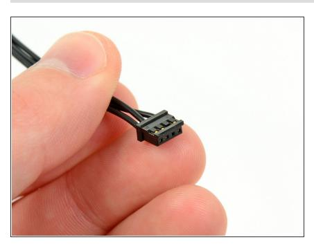
First, locate the small connector on the SSD power cable.
