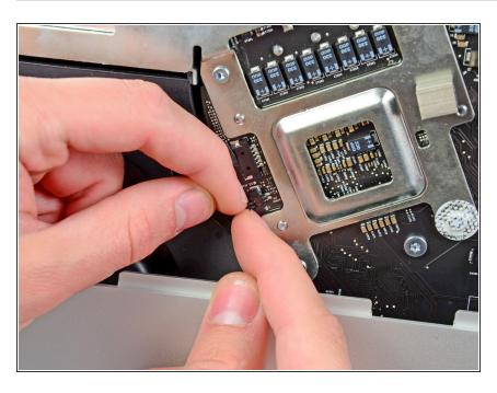
Pull the power button connector toward the bottom left corner of the iMac to disconnect it from its socket on the logic board.
