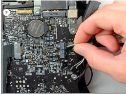
Disconnect the microphone, left speaker, and right speaker cables by pulling their connectors toward the right side of the iMac.
