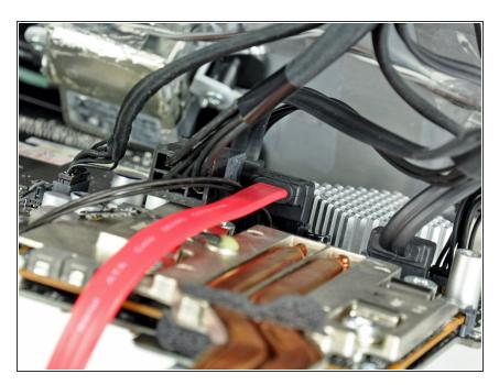
With both SATA cables connected, they should look like the logic board shown in the photo.
