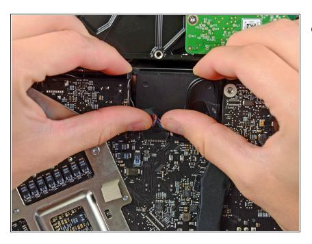
Use your thumbnails on both sides of the Bluetooth/ambient light sensor/camera/left temperature connector to push it toward the top edge of the iMac and out of its socket on the logic board.
