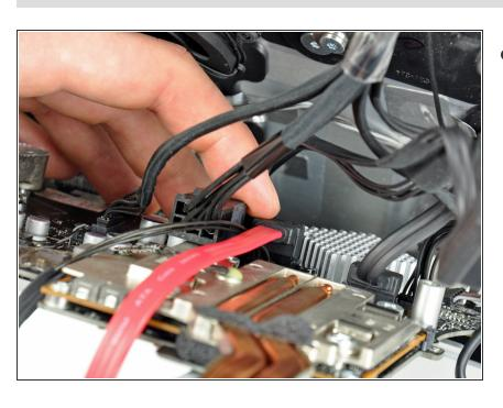
Connect the 90° end of the SATA data cable to its socket on the logic board next to the SATA power connector.
