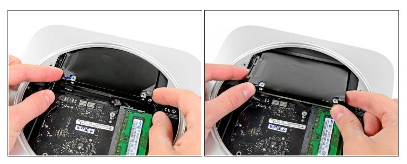
• Pull the hard drive away from the front edge of the mini and remove it from the outer case.
