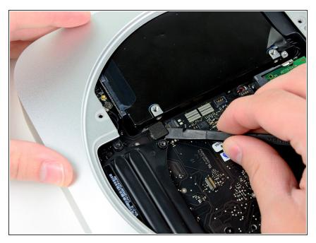
• Use the flat end of a spudger to pry the hard drive connector up from its socket on the logic board.
