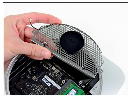
• Remove the antenna plate from the mini.
