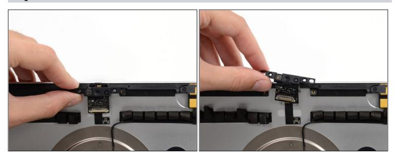
• Lift and remove the camera assembly from the iMac.
