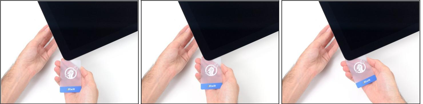
ⓘ While the opening tool cut most of the adhesive, the display will still be slightly adhered to the case. A plastic card will be necessary to free up the last of this adhesive.
