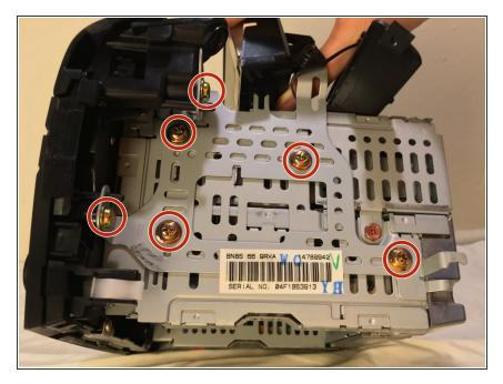
On the right side of the unit, designated by the letter R, remove 6 screws using a Phillips #2 screwdriver.
