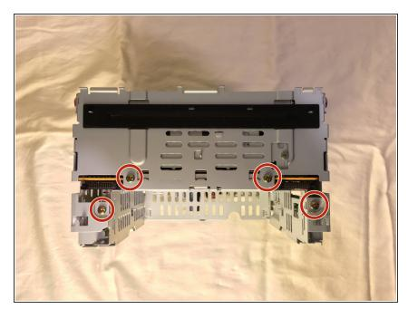
On the front of the unit, remove 4 screws with a Phillips #2 screwdriver.
