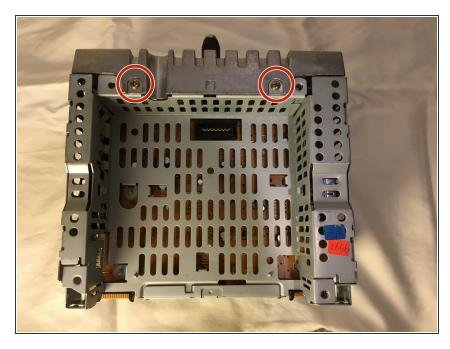
On the bottom of the unit, remove 2 screws with the Phillips #2 screwdriver.
