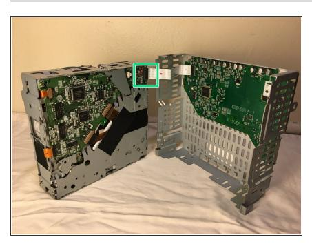
Gently pull the ribbon cable from the connector on the CD drive logic board.
