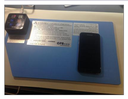
Heat the back of the phone to melt the adhesive holding the back plate on. I use an electronic heating pad, set to 60° Celsius. You can also use a heat gun, but I do not like using them. Be extra careful if using a heat gun, as they are easier to burn yourself with, and holding one over a phone for even just a little too long can damage it.
