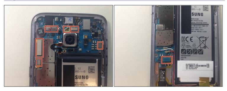
• Disconnect all other flex cables connected to the top of the logic board using the flat end of a plastic spudger.
