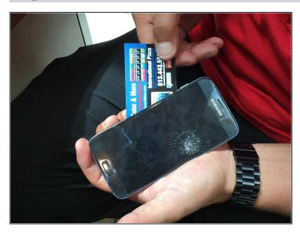
Slide a card in between the frame and display and go down slowly
