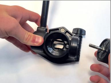
Grab the side-tilt-locking-nut with your dominant hand and grab the pan handle with your other hand. Twist the side-tilt-locking-nut counterclockwise to loosen it, and then pull it off.
