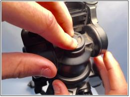
Retrieve the mounting cap and hold it on the top of the center column for 60 seconds or until it feels secure.
