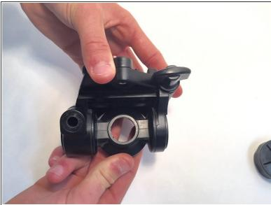
• Grab the pan head of the quick-release plate with your dominant hand and the other part of the quick-release plate with your other hand. Then, rotate the pan head clockwise 90 degrees.
