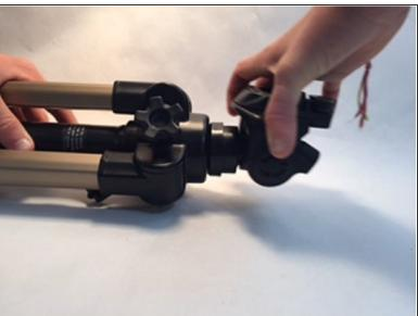
Using the more narrow part of the tripod body, place the quick-release plate back onto the tripod body.
