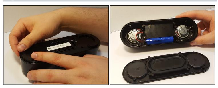
• Remove the bottom panel speaker using an iFixit opening tool.
