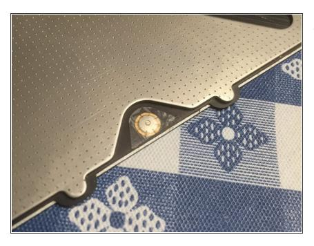
Place the tape back down and rub it with your fingernail or a plastic spudger to assure contact.
