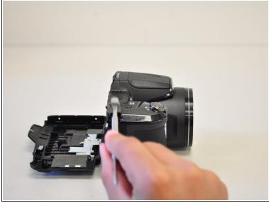
Insert a metal spludger (or another sturdy tool with a thin tip) into the hole of the lanyard ring and lift the ring upwards and out of the camera. To reassemble your device, follow these instructions in reverse order.
