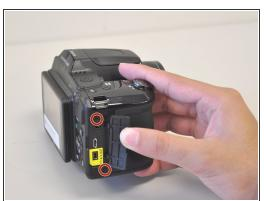
Unscrew all eight black, 4mm screws with a Philips 000. (The top-most screw shown in the third image can be accessed by lifting the cover flap off.)
